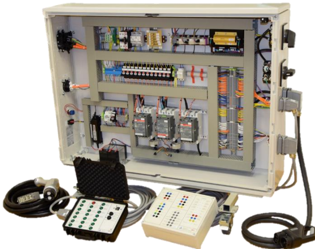
Figure 3: Measuring Distributor which can be connected between a DC-EVCS and an electric vehicle for measuring purposes as well as for initial tests (e.g. line interruptions, earth faults and short-circuits) with accessories.
